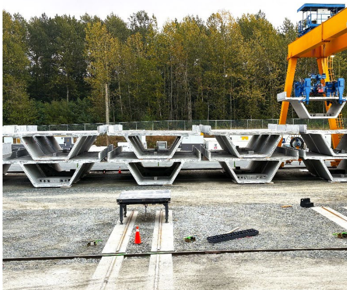
Figure 3: Stacks of precast concrete guideway segments stored at the precast concrete facility.
